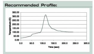
The typical profile above is designed for use with Sn10/Pb88/Ag2 or Sn5/Pb92.5/Ag2.5 alloy in a forming gas or nitrogen atmosphere (100 ppm oxygen or less). It can serve as a general guideline for establishing a profile for your process and should be regarded as a typical example. Adjustments to this profile may be necessary based on assembly size, thermal density, and other factors. Use of other alloys with lower or higher liquidus temperatures will also require changes.
