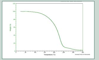
TGA was performed at a ramp rate of 10°C per minute.
