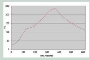
Flip-Chip Flux NC-26S is intended to be used in a nitrogen reflow environment of 100ppm oxygen or less. Some applications can utilize this material in an air environment, although best results will be obtained in an inert atmosphere. Flip-Chip Flux NC-26S can be used on many surface finishes including immersion Ag, Cu, and AuNi. These surfaces can be soldered with Pb-free alloys, but require nitrogen if reflow temperatures exceed 240°C.
