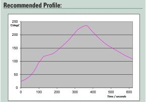
Flip-Chip Flux WS-580 is intended to be used in a nitrogen reflow environment of 100ppm oxygen or less. Some applications can utilize this material in an air environment, although best results will be obtained in an inert atmosphere. Flip-Chip Flux WS-580 can be used on many surface finishes.
