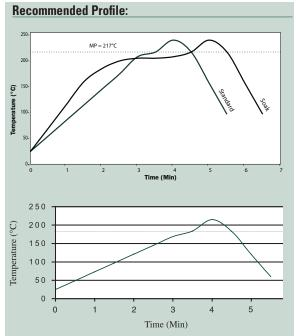
Peak reflow temperature should be <250°C in an air or nitrogen atmosphere, with a linear ramp up to approximately 30°C above the solidus temperature.
