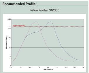
A short preheat (150°-160°C) for less than 45 seconds may be used to reduce voiding. The profile should ideally be a linear ramp at 1-2°C/second up to 20-30°C above solidus temperature, with a rapid cool down afterwards, and a minimum time above liquidus of 20 seconds.
