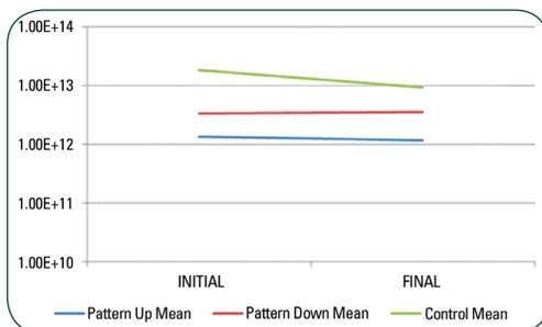
The electromigration test is performed to IPC-TM-650 method 2.6.14.1 with boards prepared using IPC-TM-650 method 2.6.3.3. The test conditions for this test are 496 hours at  $65^\circ\text{C} \pm 2^\circ\text{C}$  and 88.5%  $\pm 3.5\%$  RH. To pass this test, there should be no visible corrosion and no dendritic growth that decreases line spacing by more than 20%. In addition, the insulation resistance
