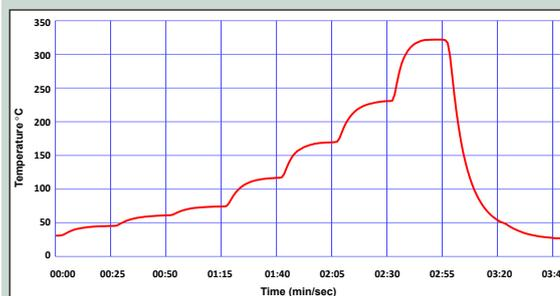
The profile above is designed for use with **BiAgX®** in a nitrogen atmosphere or forming gas (<100 ppm O<sub>2</sub>). It can serve as a general guideline for establishing a profile for your process and should be regarded as a typical example. Adjustments to this profile may be necessary based on assembly size, thermal density, and other factors.
