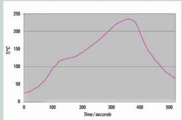
A short preheat (150°-160°C) for less than 45 seconds may be used to reduce voiding. The profile should ideally be a linear ramp at 2-3°C/second up to 20-30°C above solidus temperature, with a slow cool down afterwards of -0.5 to -0.2°C, and a minimum time above liquidus of 60 seconds.
