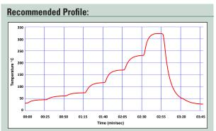
The profile above is designed for use with BiAgX® in a nitrogen atmosphere or forming gas (<100 ppm O2). It can serve as a general guideline for establishing a profile for your process and should be regarded as a typical example. Adjustments to this profile may be necessary based on assembly size, thermal density, and other factors.
