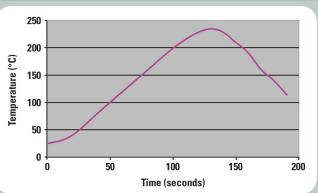
Flip-Chip Flux NC-26-A is intended to be used in a nitrogen reflow environment of 100ppm oxygen or less. Some applications can utilize this material in an air environment, although best results will be obtained in an inert atmosphere. Flip-Chip Flux NC-26-A can be used on many surface finishes including immersion Ag, Cu, and AuNi. These surfaces can be soldered with SnPb or Pb-free alloys, but require nitrogen if reflow temperatures exceed 240°C.
