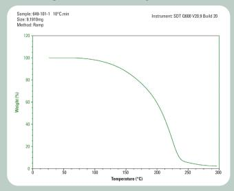
TGA was performed at a ramp rate of 10°C per minute.
