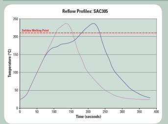
A short preheat ( $150-160^{\circ}$ C) for less than 45 seconds may be used to reduce voiding. The profile should ideally be a linear ramp at  $1-2^{\circ}$ C/second up to  $20-30^{\circ}$ C above solidus temperature, with a rapid cool down afterwards, and a minimum time above liquidus of 20 seconds.
