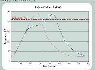
A short preheat (150–160°C) for less than 45 seconds may be used to reduce voiding. The profile should ideally be a linear ramp at 1–2°C/second up to 20–30°C above solidus temperature, with a rapid cool down afterwards, and a minimum time above liquidus of 20 seconds.
