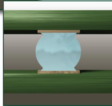
Component placement is another cause of the head-in-pillow defect. Offset placement, off-plane placement, placement pressure, and down stop, can all have a negative effect if not optimized. If the component doesn't sit down far enough and just floats on the surface of the solder paste, the spheres may not come in contact with the solder paste, dooming the process from the beginning.
