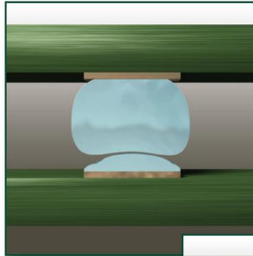
pump-out. Printing too fast or too slow will alter the amount of solder that is printed, as well as pulling the solder paste out of the apertures (scooping). Stencil design is probably the most important issue as a bad stencil
