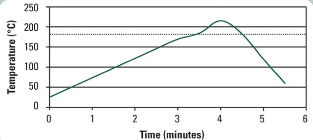
This reflow profile is designed for use with Sn63/Pb37 and Sn62/Pb36/Ag2 alloys. It will serve as a general guideline in establishing a reflow profile for this process. Adjustments to this profile may be necessary based on specific process requirements and the use of alloys with different melting temperatures.
