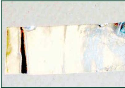
Pure indium ribbon with normal oxide layer of 80-100 Å (formed at room temperature in ambient conditions).
