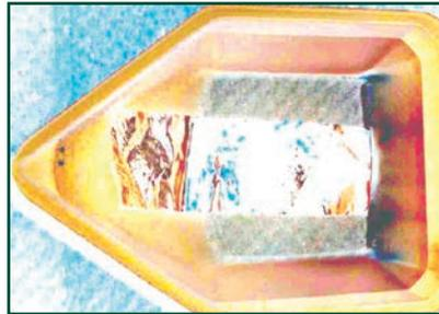
Indium ribbon being etched in the hydrochloric acid solution for 1 minute to remove oxide layer.
