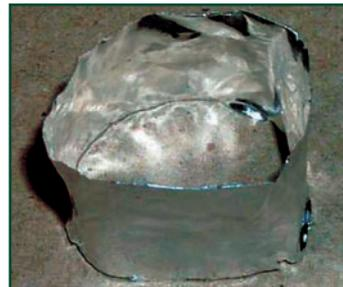
Etched indium ribbon wound back on itself and cold-welded to form a loop.
