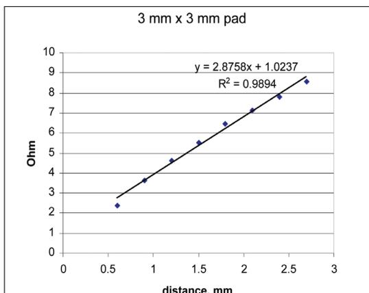
Contact resistance is calculated by multiplying the intercept (1.0237 Ohm) by the pad area (0.3cm x 0.3cm) divided by 2 (the number of pads).
